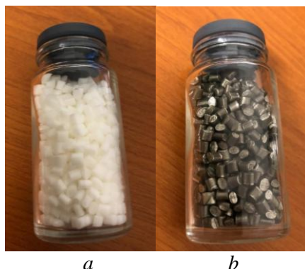
Fig. 6 – Arboblend V2 Nature granules: a ) before coating, b ) after the coating process.
