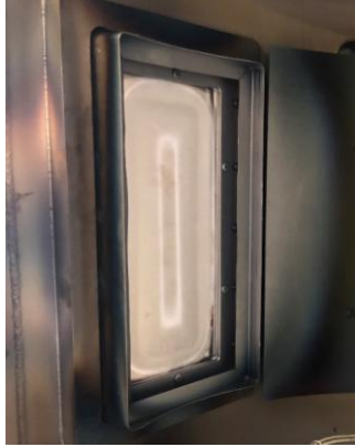
Fig. 7 – The silver source used for the nano-coating of the granules of Arboblend V2 Nature.
