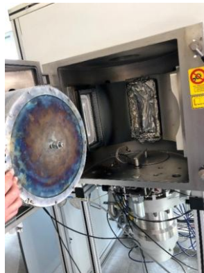
Fig. 5. The vacuum chamber of the PVD machine
