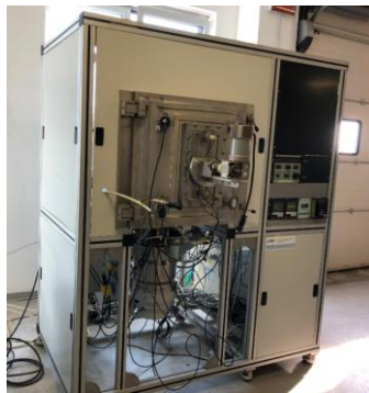
Fig. 4 – VS-40 equipment manufactured by MITEC for the physical vapor deposition (PVD) process.
